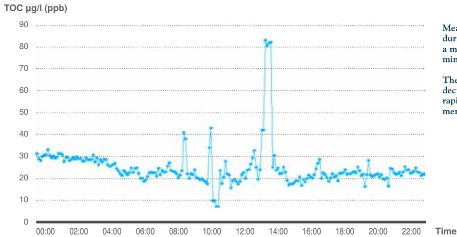
Measurement peaks during a daily cycle with a measurement cycle of 3 minutes.
